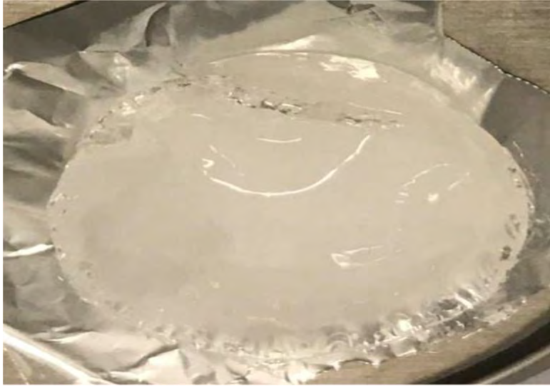
Partially disintegrated Freeze Thawed PVA gel
