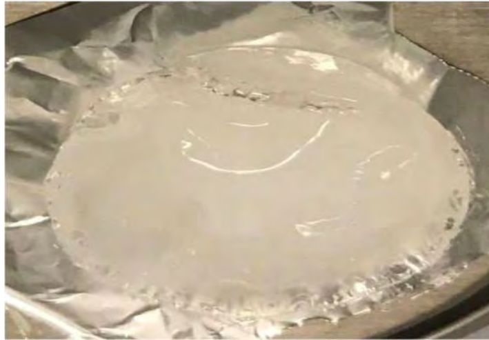
Partially disintegrated freeze-thawed PVA gel
