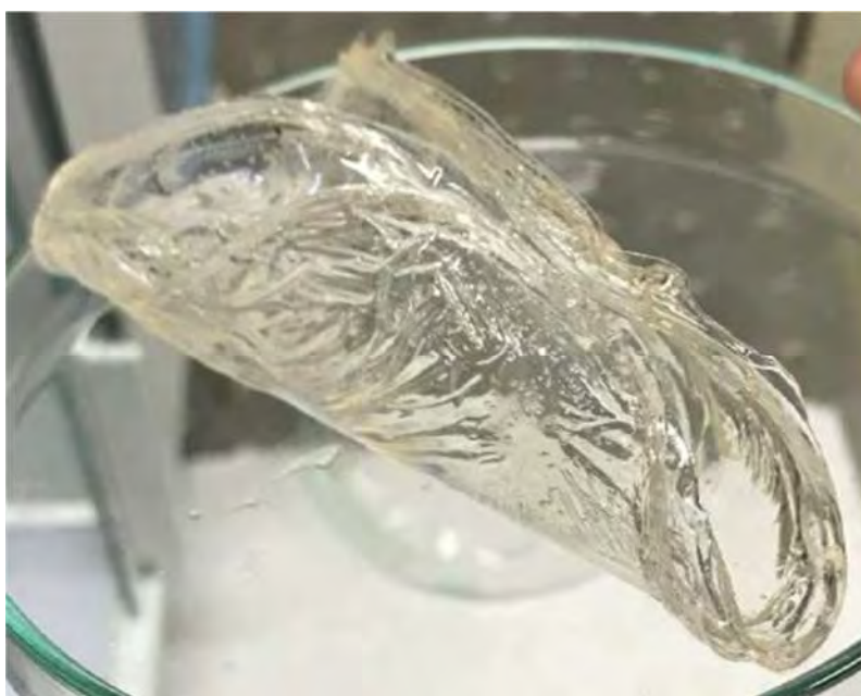
Semi-irreversible contracture of thick PVA hydrogel.
