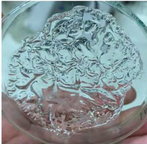
Striations on gel caused by rapid cooling and oxygen exposure of pre-gel solution.
