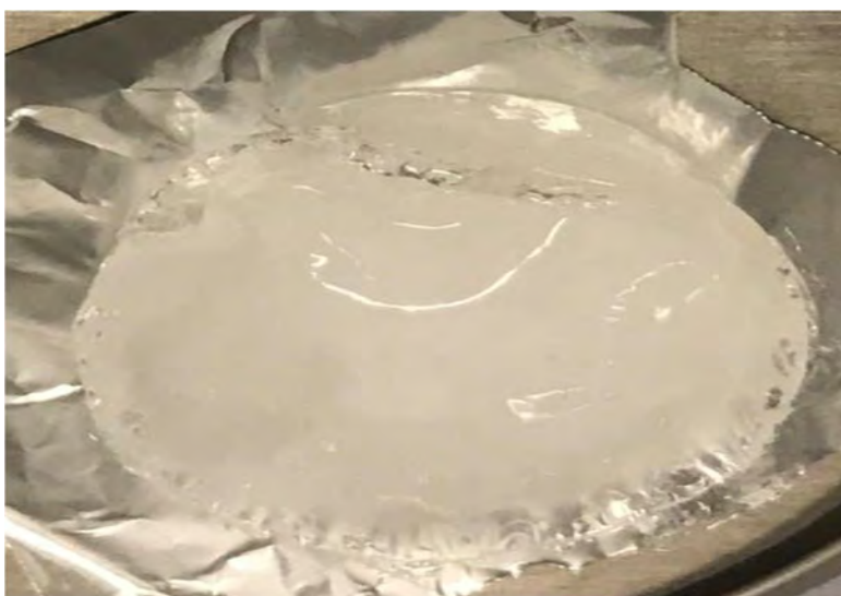
Partially disintegrated Freeze Thawed PVA gel
