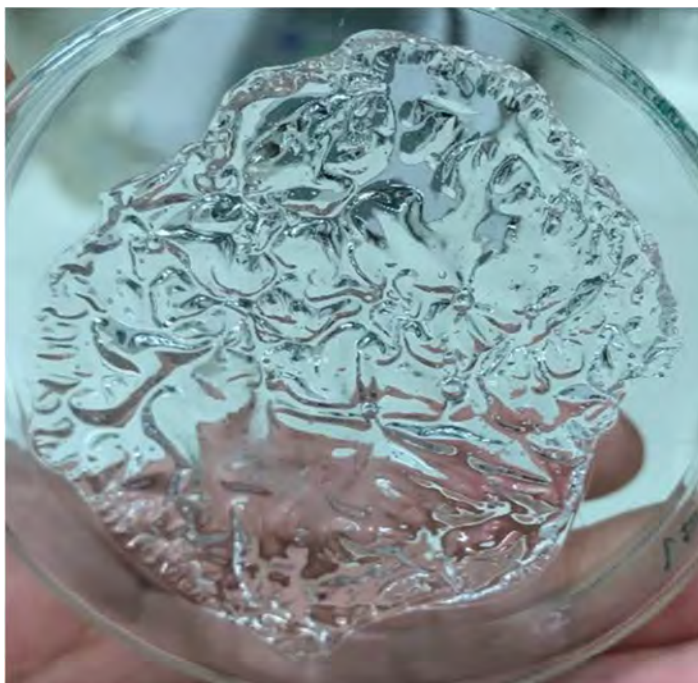
Striations on gel caused by rapid cooling and oxygenation of pre gel solution.
