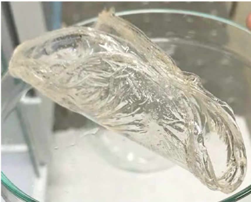
Semi-irreversible contracture of thick PVA hydrogel
