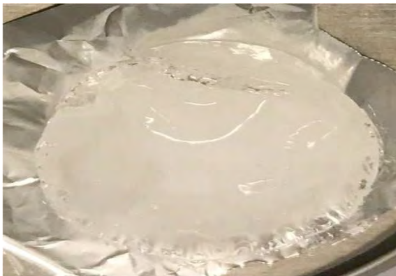
Partially disintegrated Freeze Thawed PVA gel
