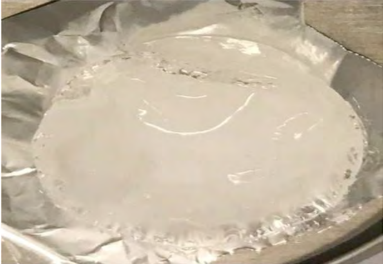
Partially disintegrated Freeze Thawed PVA gel
