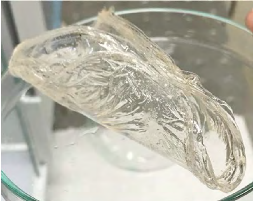
Semi-irreversible contracture of thick PVA hydrogel
