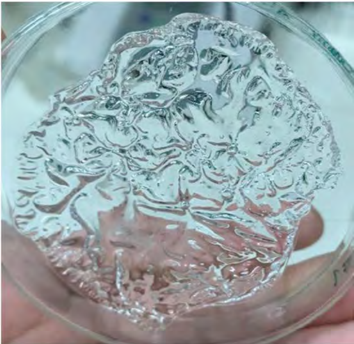
Striations on gel caused by rapid cooling and oxygenation of pre gel solution
